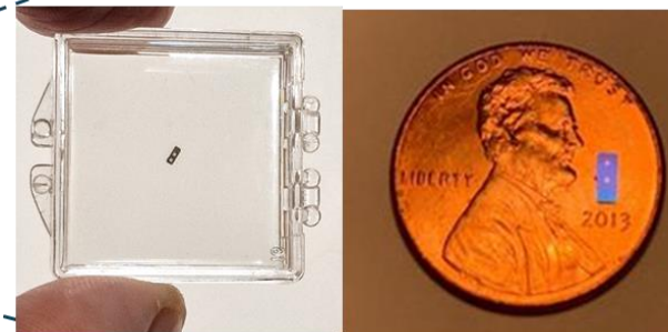
core sensor unit for human studies and CE mark chamber volume ~700 nL
